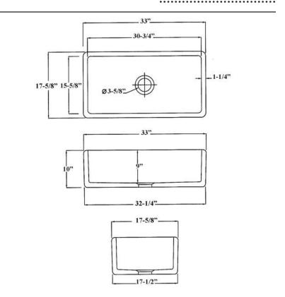
Dimensions of fixture are nominal and may vary within the range of tolerances established by ANSI Standard A112.19.2.2018 Dimensions and specifications subject to change without notice.
